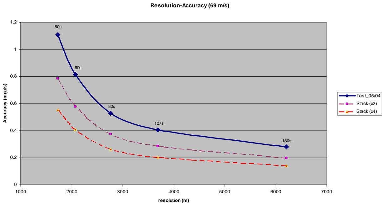
Figure 5. Accuracy-resolution graph based on five ~100 km repeat lines. The benefit of oversampling is demonstrated in curves Stack (x2) and (x4).
