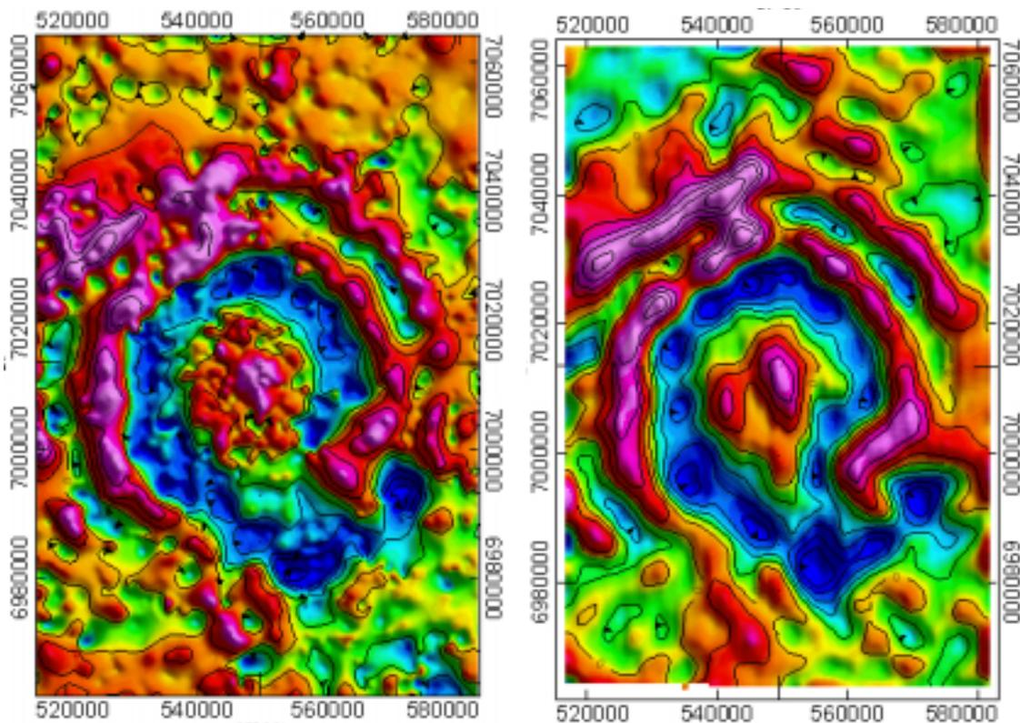
Sun-shaded upward continued First VD ground gravity
