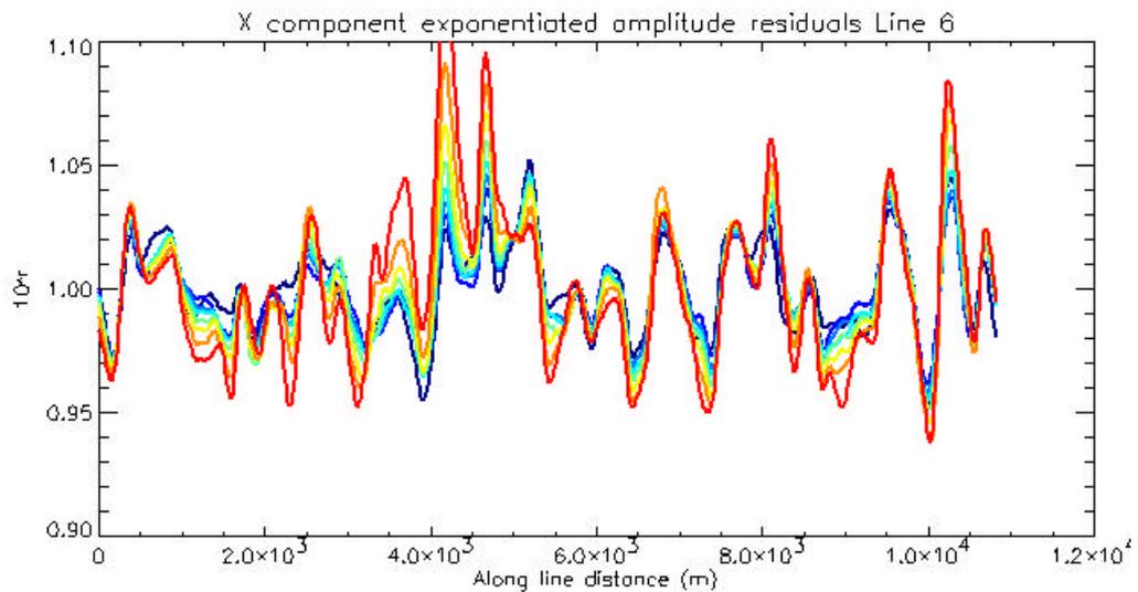
**Figure 4: Tempest Line 6 X component residuals. Early times in blue through to later times in red.**
