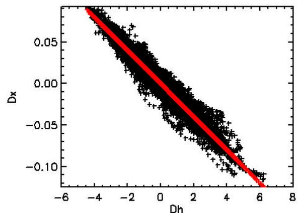
**Figure 2. Scatterplot showing the dependence of the 385Hz amplitude residuals (Dx) on flying height residuals (Dh) before "height correction".**
