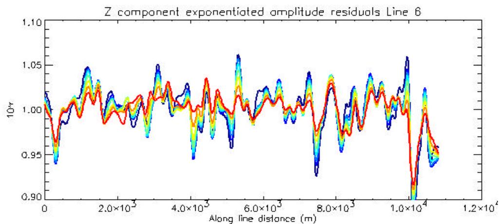
**Figure 5: Tempest Line 6 Z component residuals. Early times in blue through to later times in red.**
