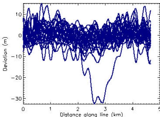
**Figure 1. Deviation from the common line for 27 Dighem flight lines**
