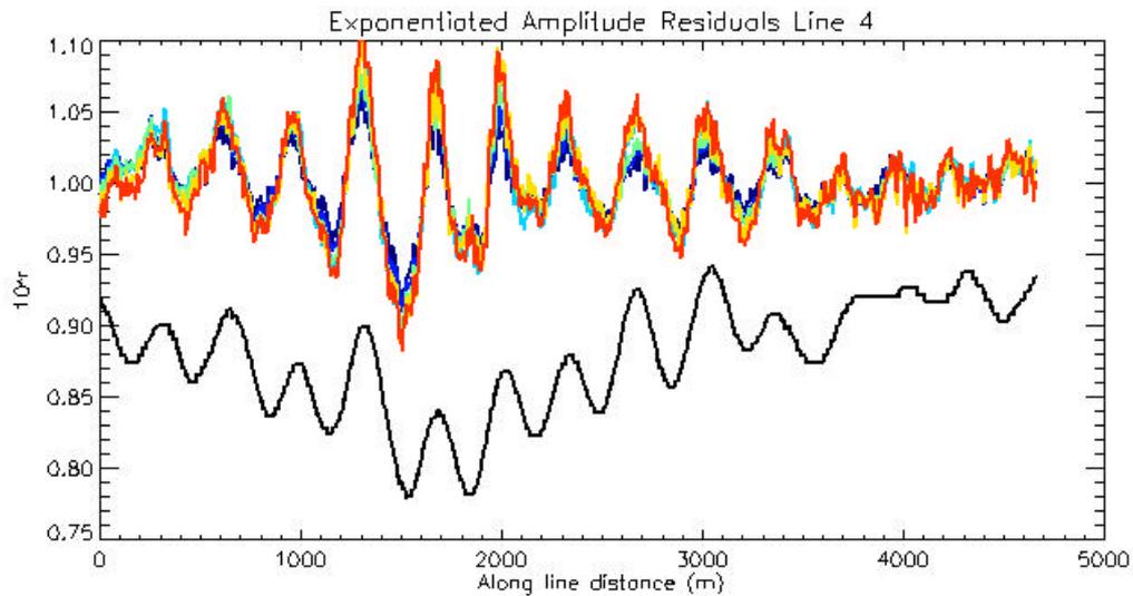
**Figure 3. Dighem Line 4 amplitude residuals for all six frequencies. High frequency in red through to low in blue. The black profile is of the transverse correction, C, required to move the observation points onto the common line (rescaled,  $C/1000 + 0.9$ ).**
